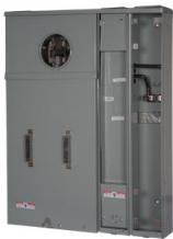
SIEMENS LOW VOLTAGE METER LOAD CENTER COMPARTMENT. MAIN LUG 4 (1 INCH) SPACES INTERIOR ALLOWING MAX 2 CIRCUITS. 4-JAW METER / 1-PHASE SYSTEM RATED 400A. SPECIAL FEATURES: OH/UG FEED, RINGLESS TYPE COVER, LEVER BYPASS SOCKET, FIELD ADDABLE SUBFEED MAIN
